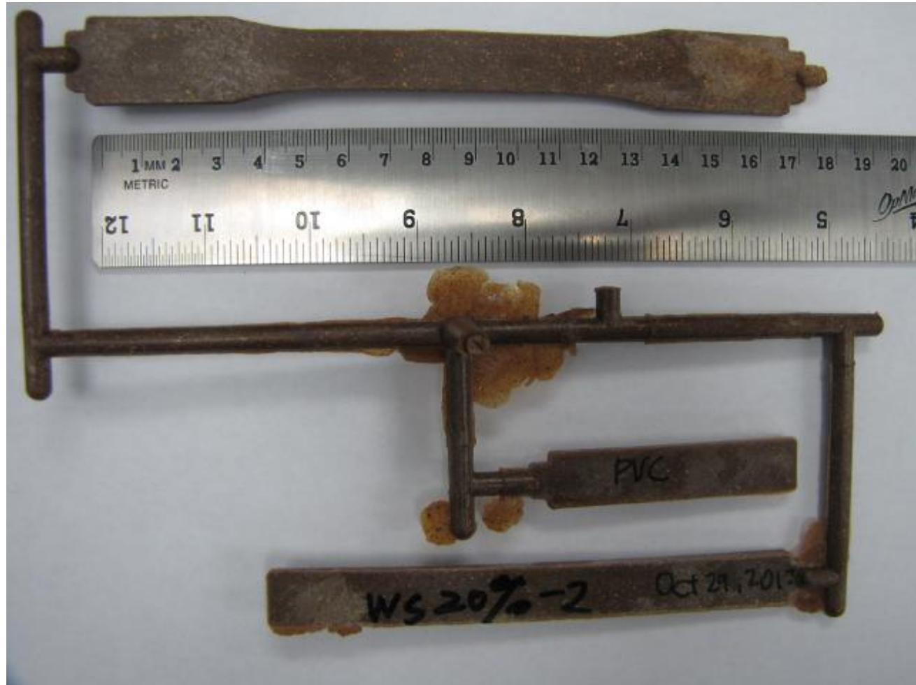
Figure 3. Test Strip produced by Injection Molding (PVC + gWSBF-25 20%-wt) . Approx. 40g.
