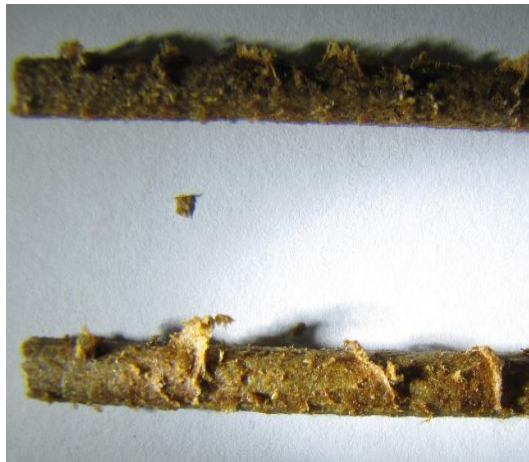
Figure 1. Extrudate 30%-gWSBF-25, ready for cutting into pellets (closeup)
