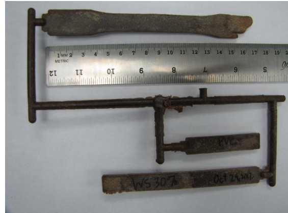
Figure 4. Test Strip produced by Injection Molding (PVC + gWSBF-25, 30%-wt) . Approx. 40 g,
