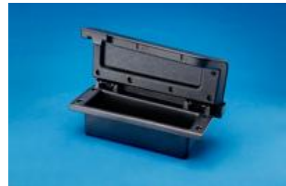
The third-row storage bins of the 2010 Ford Flex utilize a 20% wheat-straw-filled polypropylene, with the biomass increasing flexural modulus with a limited addition to part mass.
